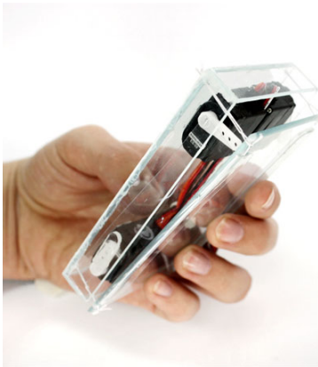
Fig. 2: Prototype. Shape-change augmented box, driven by four servo motors.
